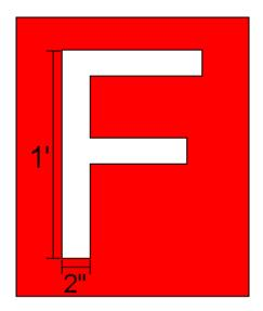
Marking: All designated fire lanes shall be marked accordingly. The perimeter of the fire lanes shall be designated by the Fire Official. All stripes shall be 5" in with. The interior of this area shall be marked with 5" yellow stripes at 45 degree angles to the perimeter strip and be 4-feet on center. All Letters shall be 1' tall and have a 2" stroke.
